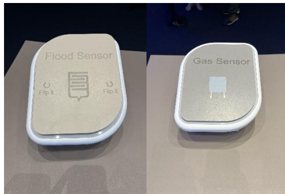
Figure 1 – Prototypes of the sensorisation solutions developed for ceramic tiles for flood and fire detection.
